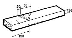
Set a marking gauge to 26mm and gauge the width of the throat on each piece, top and bottom.
