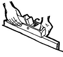
Look along the bottom of the plane to make sure the cutting edge is parallel to the sole. If one corner is too high then tap the opposite side of the blade. Repeat these actions until the plane cuts a fine, even shaving.
