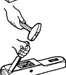
Mark radii on the top, the sides, the front, and the back of the stock. Tracing around a small tin will help to make the curves even.
