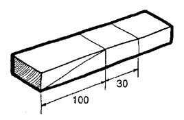
Clamp the wedge vertically in the vice and use a ripsaw to cut the angle. Plane the sawn face by clamping it in a vice horizontally, with a small piece of timber to support the thin end.
