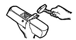
Hold the stock of the plane with one finger underneath the mouth. Put the blade into the throat and let it rest on your finger, so that it does not project below the sole of the plane. Place the wedge between the blade and the crossbar. Tap the wedge gently with a hammer to tighten it.
